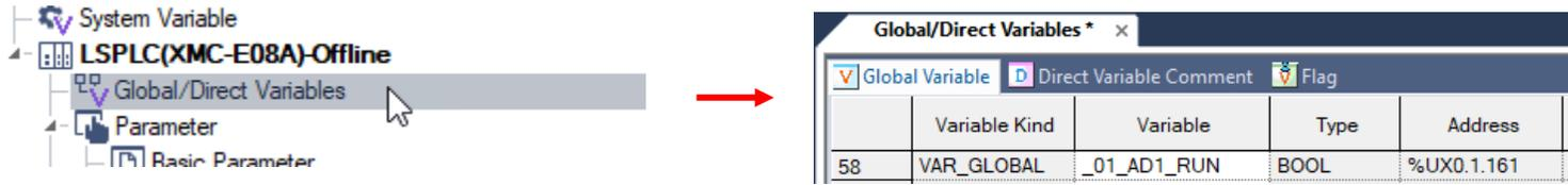
Step 4: Create a Global Variable named Port\_X0\_InputData with type Array[0...1] of BYTE. This will give us a tag with access to the input data of Port X0
