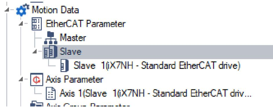
Step 7: This method will automatically connect the EtherCAT network. Go to Online Menu -> EtherCAT Slave -> Disconnect to disconnect the EtherCAT network. This will allow you to write the project to the XMC when you are ready for that.
