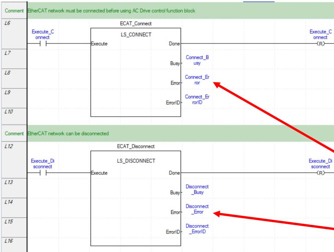
LS\_Connect must be called first to connect the EtherCAT network.
