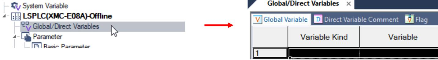
Step 4: Create some global variables to access the drive data. Below example is for reference and your variables could be named differently.
