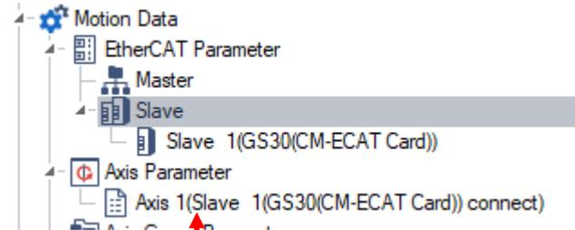
XG5000 will assign an axis to the GS30. This is done to use the LS Electric AC drive function blocks.
